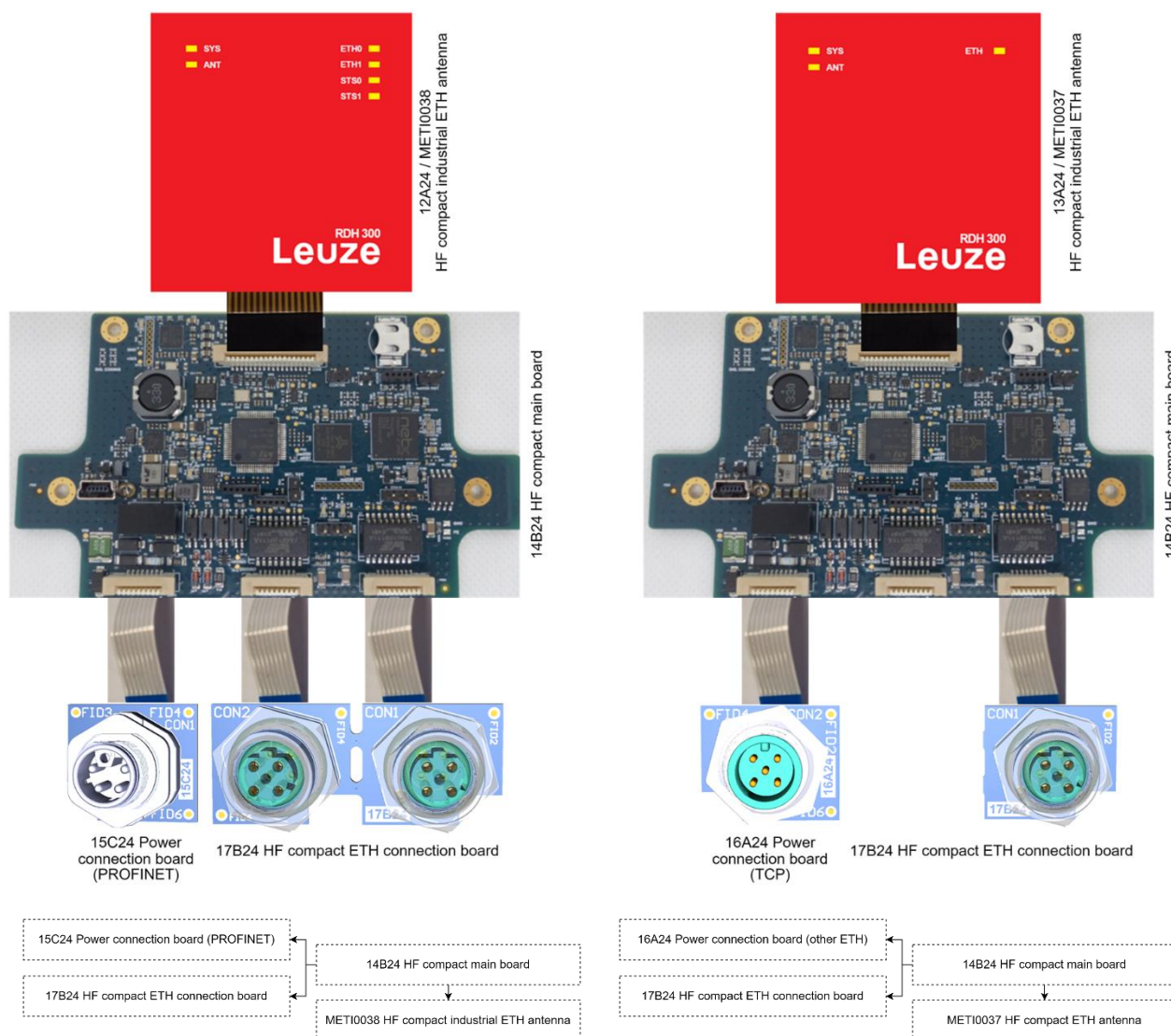
Figure 2: PCB interconnection scheme: ProfiNet (left) vs TCP (right).
